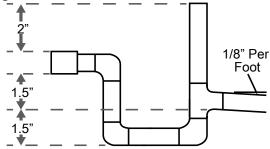
\* Some units include a painted drain connection. Using a threaded pipe or similar device to clear any excess paint accumulated inside this fitting may ease final drain line installation.
